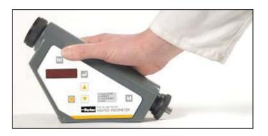
most important characteristic. It is the viscosity that gives the oil's resistance to flow and the strength of the oil film between surfaces. Viscosity can increase or decrease as a result of problems such as contamination, fuel dilution, and shear thinning. Measurement of viscosity is extremely important for hydraulic oils, diesel engine oils, gear, and fuel oils.
