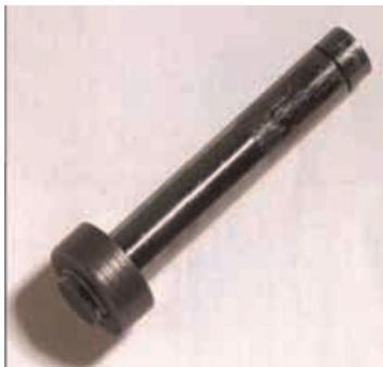
Injector plunger scuffing and seizure is nearly always caused by excessive amounts of water in the fuel.
